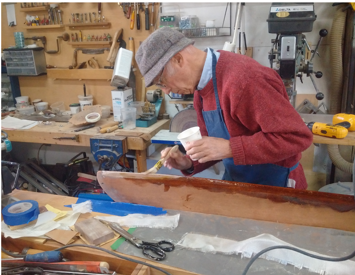
Tom applying epoxy to reinforce centreboard edge with a layer of fiberglass
