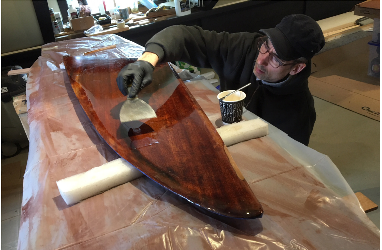
Christopher applying epoxy resin to the centreboard
