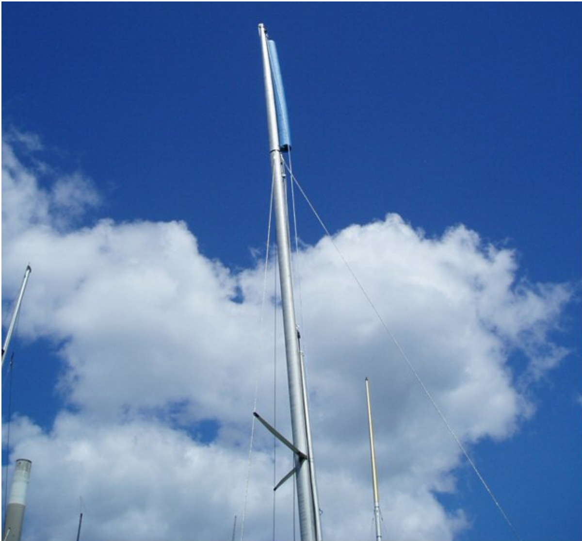
Masthead floatation before initial test
