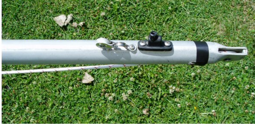
Masthead pad eye and block below wind indicator fitting
