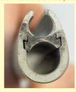
and is hollow in the centre to house the supplied forestay, which is enclosed in a plastic sleeve, thus isolating it from the spar, avoiding galvanic corrosion, and maintaining a tight fit, which also contributes to the overall stiffness of the spar. The rear part of the spar slides into the front part and has a concave slot at the back to hold the leading edge of the sail. When fully assembled the two sections of the spar together measure 23.5mm from front to back. The slim nature
