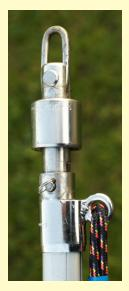
the halyard.) A good quality swivel is important in any furling or reefing system, but some of the cheaper versions are not really up to the job and tend not to work properly under load. This one is engineered to work well under load, and does so. As with the drum, the swivel supplied in this system could be used as part of a non-reefing furling system with a view to a subsequent upgrade.
