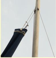
Incidentally, the aluminium profile only comes in lengths up to 2m, so obviously the spar has to be supplied in several lengths. They are pre-cut to the exact total length required to match the supplied forestay, and cannot be shortened without replacing the forestay.
