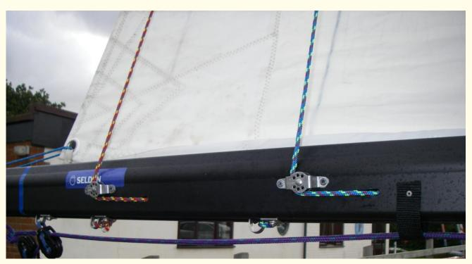
efficient method is to thread shock cord through the sail from front to back with hooks secured on it so the cord can be hooked together under the boom thus securing the loose sail.
