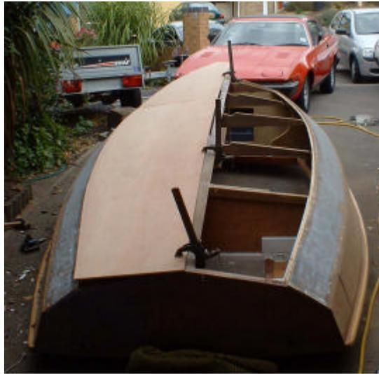
Remove the keel to locate the screws. Endeavour to remove the keel in as few pieces as possible. If it breaks, I'll tell you how to make another one. Remove the keel, not the screws that attach the floor supports and make a nice oversized one as described above.
