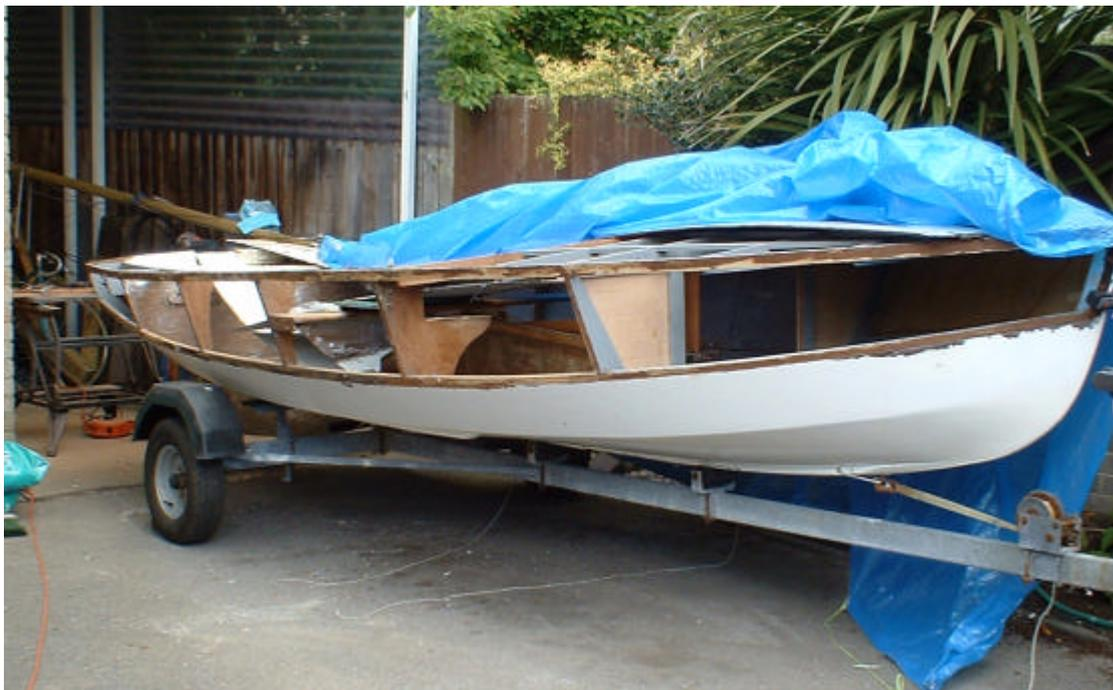
Replacement is more work, though easier if you got the old panel off in one piece. The topside panel is made from 3 pieces of plywood
