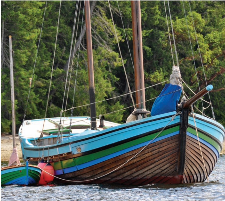
ABOVE— This colourful clinker-built ketch at Manson's Landing is based on a 1700s Finnish coastal freighter.
